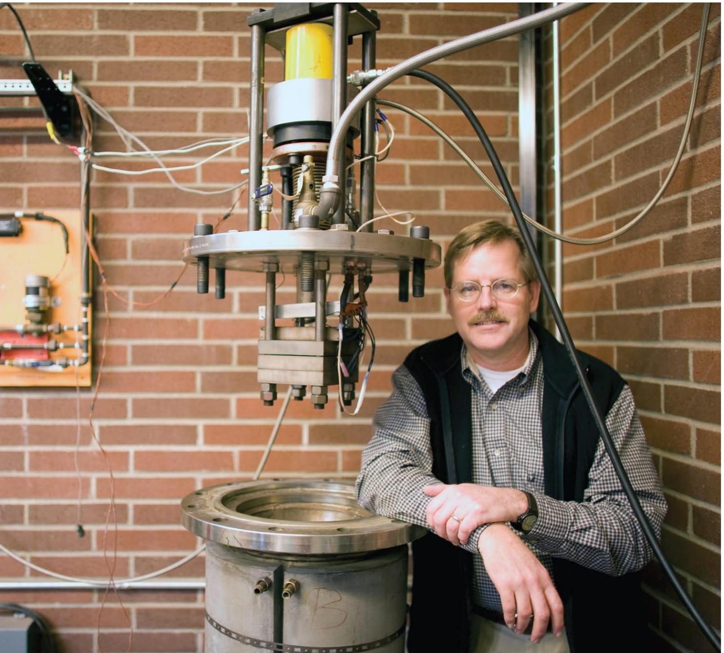
*Fred Kamke, standing next to a device he developed to manufacture viscoelastic thermal compression (VTC) wood specimens. The device is used to make test specimens for evaluation. Photo courtesy of University Advancement.*
